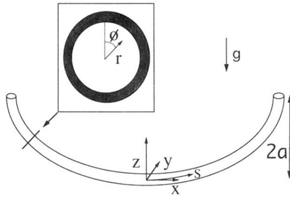
FIG. 2. Coordinate system used for cycloidal tube geometry. The longitudinal coordinate, along the fiber's axis, is  $s$ . The inset is a cross section through the fiber showing the transverse polar coordinates  $r$  and  $\phi$  which are centered on the fiber axis. The fiber bent into a gravitational cavity is shown schematically. The height of the cycloid is  $2a$ .
