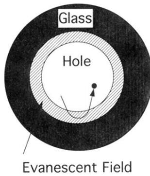
FIG. 1. Schematic cross section of a hollow optical fiber. The glass (shading) is the optical waveguide while the hole is the atomic pipe or waveguide. The atoms are confined transversely by the evanescent light field (hatching) at the glass-hole interface. A schematic trajectory of an atom (black disk) reflected by the evanescent light field is shown. As in conventional fibers the glass may be doped to form a high refractive index light guiding region adjacent to the hole.
