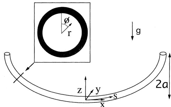
FIG. 2. Coordinate system used for cycloidal tube geometry. The longitudinal coordinate, along the fiber's axis, is  $s$ . The inset is a cross section through the fiber showing the transverse polar coordinates  $r$  and  $\phi$  which are centered on the fiber axis. The fiber bent into a gravitational cavity is shown schematically. The height of the cycloid is  $2a$ .
