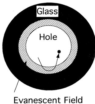
FIG. 1. Schematic cross section of a hollow optical fiber. The glass (shading) is the optical waveguide while the hole is the atomic pipe or waveguide. The atoms are confined transversely by the evanescent light field (hatching) at the glass-hole interface. A schematic trajectory of an atom (black disk) reflected by the evanescent light field is shown. As in conventional fibers the glass may be doped to form a high refractive index light guiding region adjacent to the hole.
