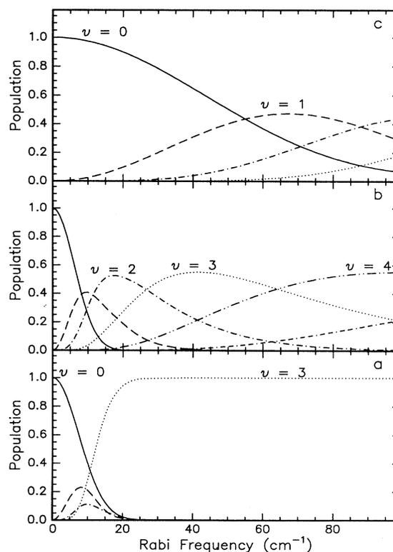
FIG. 3. Rabi frequency (peak) dependence of each of the wave forms described in Eq. (6). (a) Complex hyperbolic secant  $\tau_p = 4 \text{ ps}$ ,  $\mu = 14.2$ ; (b) linearly swept hyperbolic secant  $\tau_p = 4 \text{ ps}$ ,  $b = 9.4 \text{ cm}^{-1}/\text{ps}$ ; and (c) unmodulated hyperbolic secant  $\tau_p = 150 \text{ fs}$ .  $v=5$  (— · — · —); others as labeled. The pulse center frequency is  $2125 \text{ cm}^{-1}$  in (a) and (c);  $2147 \text{ cm}^{-1}$  in (b).
