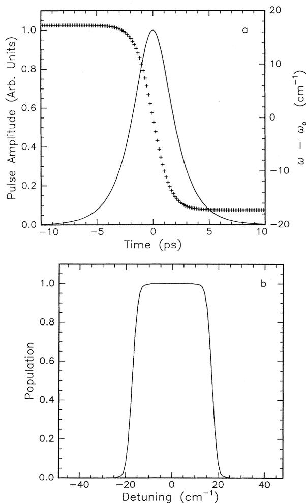
FIG. 1. (a) Pulse amplitude profile (—) and corresponding hyperbolic tangent frequency sweep (++++) of the pulse  $\epsilon(t) = \text{sech}(\alpha t)^{1+5i}$ . The pulse width  $\tau_p$  (FWHM) is 4 ps. (b) The near-rectangular inversion spectrum produced by the pulse in (a) for a two-level system with a peak Rabi frequency of  $2\pi \times 50 \text{ cm}^{-1}$ .
