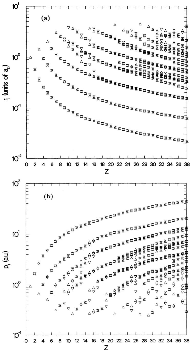
FIG. 5. (a) Distances  $r_i$  from the nucleus and (b) momenta  $p_i$  of quasiclassical electrons in the ground-state configuration,  $i = 1$  to  $Z$ . Upward (downward)-pointing triangles are for  $\alpha$  ( $\beta$ )-spin electrons.
