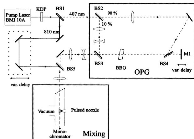
FIG. 1. Experimental setup. The radiation of the Ti:sapphire pump laser is frequency doubled. The second harmonic is separated and used to pump an optical parametric generator (OPG). The fundamental radiation and the tunable radiation from the OPG are mixed in the gas jet of the pulsed nozzle.
