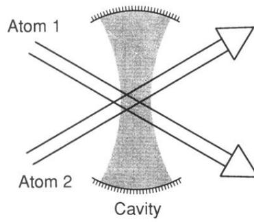
FIG. 1. Proposed configuration for the preparation of the entangled state (singlet state) of two two-level atoms. Initially the cavity is in the vacuum state. Atom 1 enters the cavity in its excited state and atom 2 in its ground state. After crossing the cavity, the atoms become entangled and the cavity is left in its original state: the vacuum.
