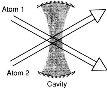
FIG. 1. Proposed configuration for the preparation of the entangled state (singlet state) of two two-level atoms. Initially the cavity is in the vacuum state. Atom 1 enters the cavity in its excited state and atom 2 in its ground state. After crossing the cavity, the atoms become entangled and the cavity is left in its original state: the vacuum.
