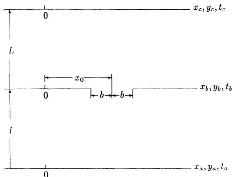
FIG. 1. The geometry of the single-slit diffraction experiment. The slit at  $y_b$  has width  $2b$  and is centered at  $x_b = x_0$ . The distances  $l$  and  $L$  are given by Eqs. (2.6) and (2.7), respectively.
