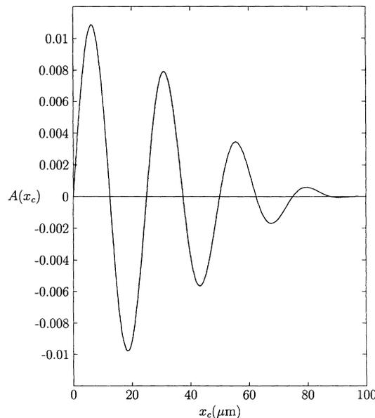
FIG. 4. The asymmetry in the two-slit diffraction pattern as in Fig. 3 but with electron wavelength  $\lambda = 5 \times 10^{-5} \text{ } \mu\text{m}$ . Here the approximate and the exact results coincide.
