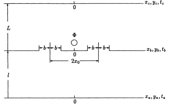
FIG. 2. The geometry of the two-slit diffraction experiment. Magnetic flux  $\Phi$  is present in a shielded solenoid at  $x_b = 0$ . The slits of width  $2b$  are centered at  $\pm x_0$ , and are separated by a distance  $2x_0$ . The distances  $l$  and  $L$  are given by Eqs. (2.6) and (2.7), respectively.
