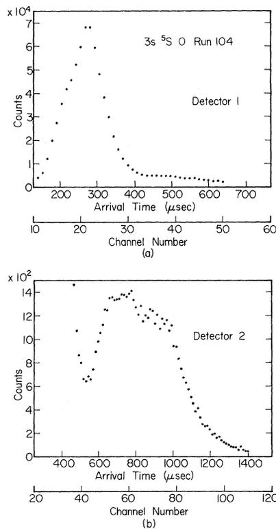
FIG. 1.  $O(^5S)$  time-of-flight distributions, representing about  $10^6$  separate data-collection sweeps. The tail of a large peak appearing in the first few channels of the detector-2 distribution represents neutral atoms or molecules with kinetic energies greater than 20 eV; they result from the acceleration of either  $O^+$  or  $O_2^+$  ions in the electron gun followed by charge exchange in the source chamber region.
