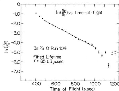
FIG. 2. Decay plot. The ratio of detector-2 to detector-1 metastable atom time-of-flight distributions is a straight line on a logarithmic plot. The measured lifetime  $\tau$  is obtained from the slope ( $= -1/\tau$ ) of the least-squares-fitted straight line.
