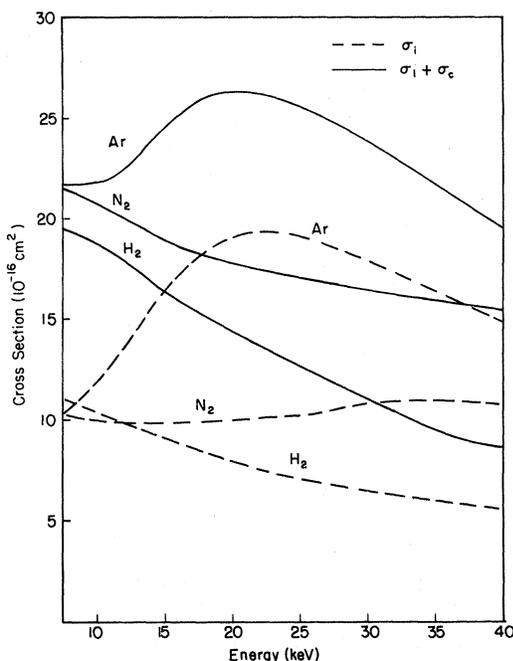
FIG. 2. Plots of the computed  $n=3$  collisional ionization cross sections and the sum of these ionization cross sections and the cross sections for electron capture. This sum should be a good approximation for the destruction of all excited states.
