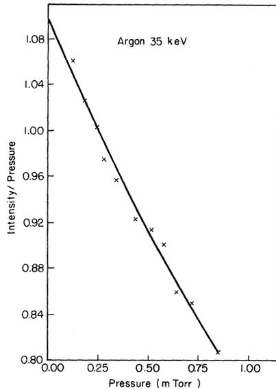
FIG. 1. Intensity per unit pressure of the  $3s \rightarrow 2p$  radiation as a function of the collision chamber pressure. The target gas is argon. The line is a computer fit of Eq. (1) to the data points using  $Q_i$  as the fitting parameter.
