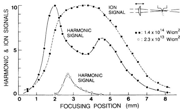
FIG. 9. The ninth-harmonic and ion signals in Xe as a function of position of the (616-nm) dye-laser focus at the intensity  $I = 1.4 \times 10^{14}$  W/cm<sup>2</sup> (solid circle and square) and  $2.3 \times 10^{13}$  W/cm<sup>2</sup> (open circle). The maximum harmonic and ion signals are normalized to 10. The confocal parameter  $b = 8.0$  mm.
