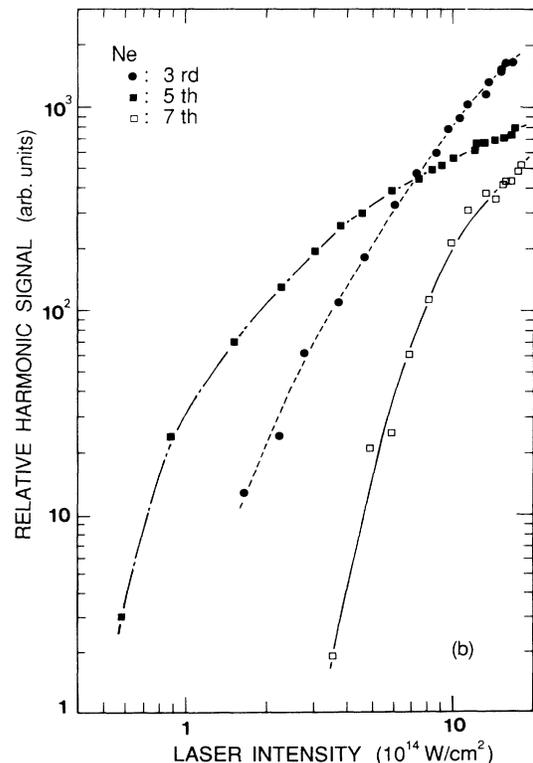
FIG. 7 The third-, fifth-, and seventh-harmonic signals in (a) He and (b) Ne as a function of the XeCl laser intensity.
