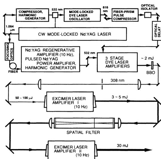
FIG. 1. Experimental arrangement of the subpicosecond XeCl laser amplification system. The UV laser is based on a sub-ps dye-laser oscillator-amplifier system of which output wavelength is tuned to 616 nm. BBO denotes a  $\beta$ -BaB<sub>2</sub>O<sub>4</sub> crystal.
