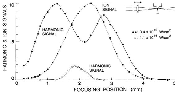
FIG. 6. The fifth harmonic and ion signals in He as a function of position of the XeCl laser focus at  $I = 3.4 \times 10^{15}$  W/cm<sup>2</sup> (solid circle and square) and  $I = 1.1 \times 10^{14}$  W/cm<sup>2</sup> (open circle). The maximum harmonic and ion signals are normalized to 10. The confocal parameter  $b = 4.5$  mm.
