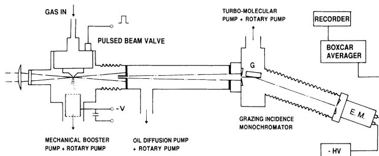
FIG. 2. Experimental arrangement for the harmonic generation. E.M., Electron multiplier; G, Grating.
