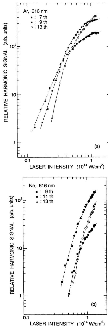
FIG. 8. Harmonic signals in (a) Ar and (b) Ne as a function of the (616-nm) dye-laser intensity.
