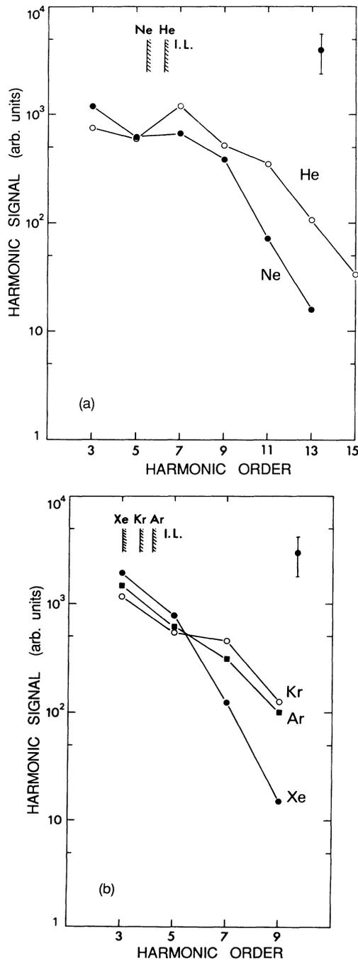
FIG. 4. Harmonic distributions observed in (a) He at  $I = 2.5 \times 10^{15}$  W/cm<sup>2</sup> and Ne at  $I = 2.8 \times 10^{15}$  W/cm<sup>2</sup>, and (b) Ar, Kr, and Xe at  $I = 3.1 \times 10^{15}$  W/cm<sup>2</sup> with the XeCl laser pulses. IL denotes the ionization limit.
