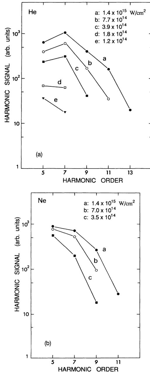
FIG. 5. Harmonic distributions for (a) He and (b) Ne at several XeCl laser intensities.
