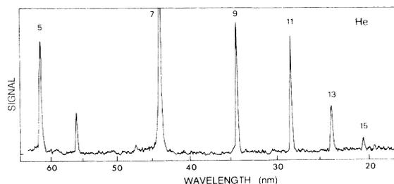
FIG. 3. Example of the high-order harmonic spectrum observed in He at the XeCl laser intensity  $I = 2.5 \times 10^{15} \text{ W}/\text{cm}^2$  with the grazing-incidence monochromator. The spectral peaks are labeled by the harmonic order, whereas the unmarked peaks are the second-order diffractions from the grating.
