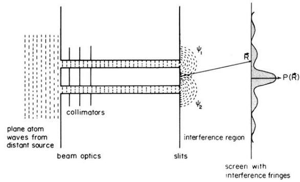
**FIG. 1.** Two-slit experiment with atoms. A set of wider slits collimates two atom beams which illuminate the narrow slits where the interferences pattern originates.
