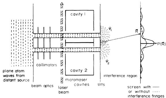
FIG. 2. Two-slit interference pattern at a screen associated with the state of a micromaser *Welcher-Weg* detector setup. The setup of Fig. 1 is supplemented by two high-quality micromaser cavities and a laser beam to provide which-path information. This is accomplished by arranging things such that every time an atom passes through the pair of micromaser cavities it leaves a photon in one or the other cavity, thus providing which-path information, see Ref. [7].
