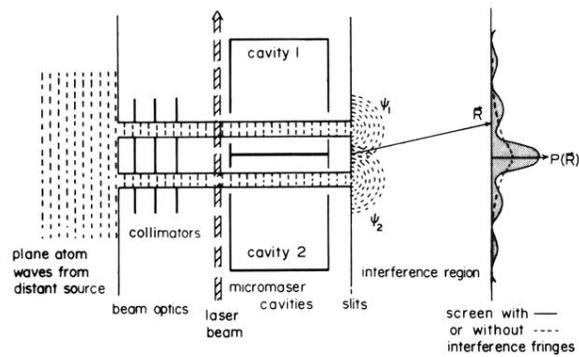
FIG. 2. Two-slit interference pattern at a screen associated with the state of a micromaser *Welcher-Weg* detector setup. The setup of Fig. 1 is supplemented by two high-quality micromaser cavities and a laser beam to provide which-path information. This is accomplished by arranging things such that every time an atom passes through the pair of micromaser cavities it leaves a photon in one or the other cavity, thus providing which-path information, see Ref. [7].
