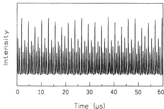
FIG. 4. Typical intensity variation for period-doubling chaos of the laser: pump intensity,  $4.6 \text{ W/cm}^2$ ;  $\text{NH}_3$  gas pressure,  $7.5 \text{ Pa}$ .
