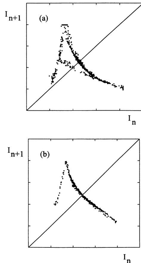
FIG. 7. First-peak-intensity return map constructed from the type-III intermittency of the laser: (a) under the influence of the pump-coherence effects of the laser and (b) under the condition that the pump-coherence effects can be neglected.
