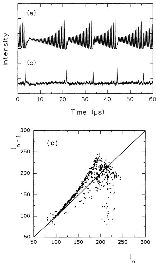
FIG. 3. Influence of weak counterpropagating emission on the Lorenz-type dynamics of the laser spiral chaos: (a) typical intensity of the laser spiral chaos in the presence of the forward emission, (b) intensity variation of the forward emission, and (c) first-peak-intensity return map constructed from the laser spiral chaos shown in (a).
