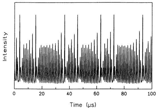
FIG. 6. Typical intensity variation for type-III intermittency of the laser: pump intensity,  $7 \text{ W/cm}^2$ ;  $\text{NH}_3$  gas pressure, 4 Pa.
