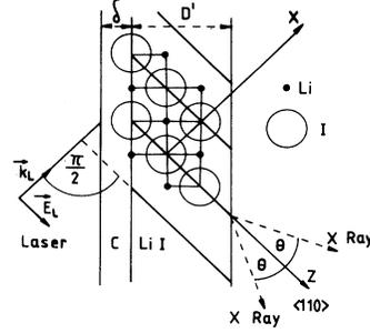
FIG. 2. The scheme of the experimental arrangement proposed.  $k_L$  and  $E_L$  are the wave vector and the electric field strength of the laser radiation,  $\delta$  and  $D'$  are the widths of the graphite layer and the LiI crystal ( $D = 2^{1/2}D'$ ). The other notation is the same as in Fig. 1.
