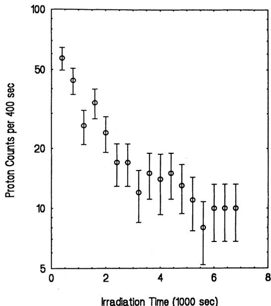
FIG. 2. Integrated fusion proton counts per 400 sec as a function of beam exposure time of a PDE target. The results were obtained with a 1-nA (D<sub>2</sub>O)<sub>5</sub>D<sup>+</sup> cluster-ion beam accelerated at 638 keV.
