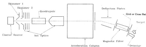
FIG. 1. Schematic diagram of the experimental apparatus (not to scale).
