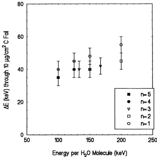
FIG. 6. Energy loss in 10  $\mu\text{g}/\text{cm}^2$  carbon films of various water clusters containing up to five molecules plotted as a function of energy per molecule. The cluster ions have the formula  $(\text{H}_2\text{O})_n\text{H}^+$ .
