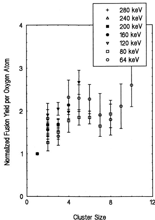
FIG. 5. Knock-on fusion yields per oxygen atom of  $\text{H}_2\text{O}$  clusters normalized to the yields of  $\text{H}_3\text{O}^+$  at various energies per oxygen atom as a function of the cluster size.
