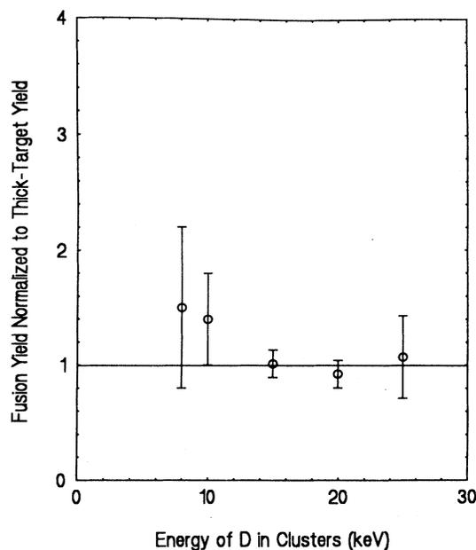
FIG. 3. Fusion yields of small D<sub>2</sub>O clusters incident on D<sub>2</sub>O ice, normalized to thick-target yields. The yields were measured with clusters containing 1–7 D<sub>2</sub>O molecules and corrected for oxygen knock-on yields.
