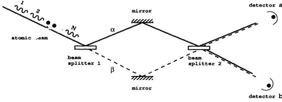
FIG. 2. We illustrate a scheme whereby a stream of  $N$  atoms are sent through a simple interferometer during a measurement time  $t_m$ . The atoms are split at beam splitter 1, follow paths  $\alpha$  or  $\beta$ , are reflected off the mirrors, and are then recombined at beam splitter 2. The recombined atoms are detected at upper detector  $a$  or lower detector  $b$  where interference fringes are recorded.
