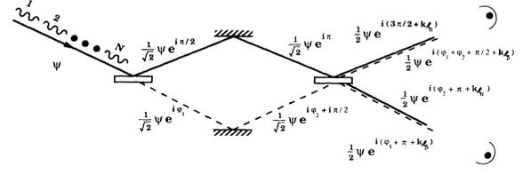
FIG. 3. Chasing phases through the interferometer accounts for accumulated phase shifts in the upper or lower branches. The phase shift upon reflection is arbitrary, but we choose it here to be  $\pi/2$  for simplicity. Upon transmission, a phase shift of  $\varphi_1$ , or  $\varphi_2$ , is assumed for beam splitter 1 or 2, respectively
