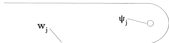
FIG. 6. A wake w_j of excited and ionized atoms is produced by each packet \psi_j . Droplets condense on the ions to form a visible track.
