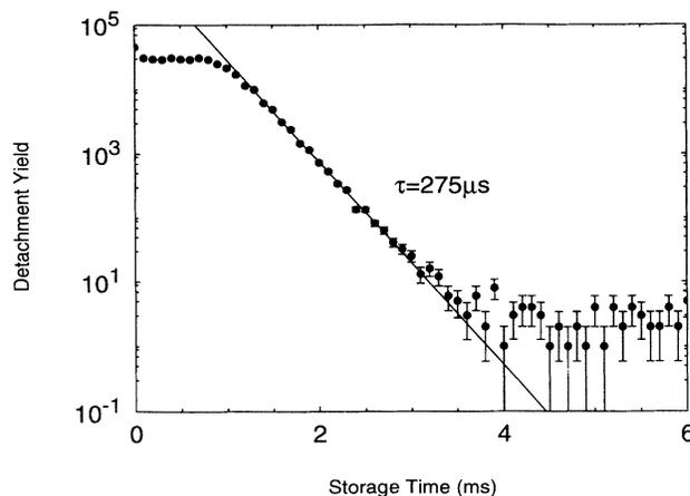
FIG. 3. Typical neutral-atom signal from tandem-channel-plate detector as a function of time following ion-beam injection.
