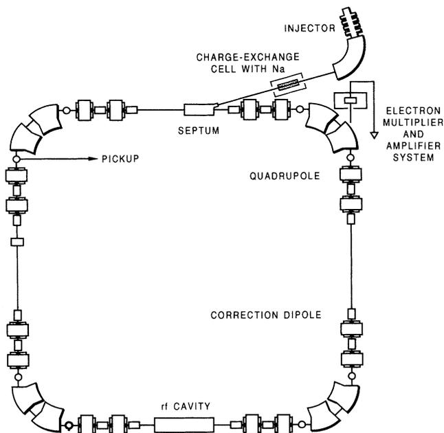
FIG. 2. The storage-ring setup, showing ion injector, charge-exchange facility, and the particle-detection system.
