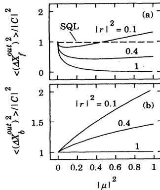
FIG. 2. Variance in the quadrature components of the output fields as functions of the phase-conjugate reflectivity  $|\mu|^2$  for various mirror reflectivities (a) on the side of the phase-conjugate mirror, and (b) on the side of the ordinary mirror. The variances are normalized to the standard quantum-noise limit (SQL).
