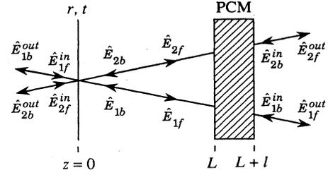
FIG. 3. Schematic illustration of the phase-conjugate resonator and the off-axis fields.
