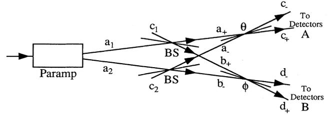
FIG. 1. Schematic diagram of the transformations involved in the experimental arrangement to test Bell's inequalities (BS denotes beam splitter).
