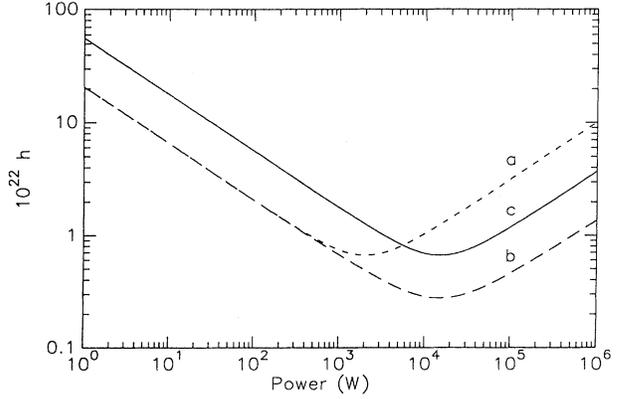
FIG. 7. A comparison between using (curve  $a$ )  $\theta=0$  and (curve  $b$ )  $\theta^{\text{opt}}$ , in the calculation for the minimum possible value of  $h$  detectable using  $r=1$ . The corresponding curve for no squeezing ( $r=0$ ) is also shown (see curve  $c$ ).
