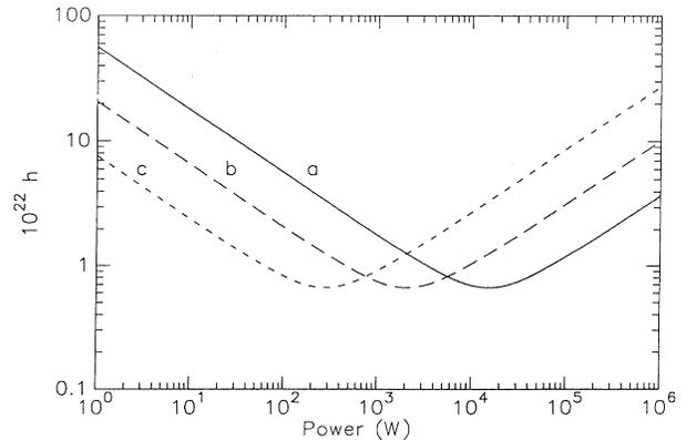
FIG. 5. The minimum possible gravitational wave amplitude  $h$  detectable as a function of power using  $\theta=0$ , for three different values of the squeezing parameter  $r$ : (curve a)  $r=0$ , (curve b)  $r=1$ , (curve c)  $r=2$ .
