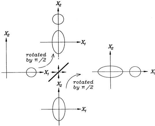
FIG. 4. Amplitude squeezed light on the outside looks like phase squeezed light inside the cavities.
