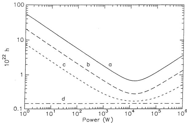
FIG. 6. The minimum possible value of  $h$  detectable as a function of power using  $\theta^{\text{opt}}$ , for three different values of the squeezing parameter  $r$ : (curve  $a$ )  $r=0$ , (curve  $b$ )  $r=1$ , (curve  $c$ )  $r=2$ . The contribution of the mirror noise to  $h$  has also been drawn in (see curve  $d$ ).
