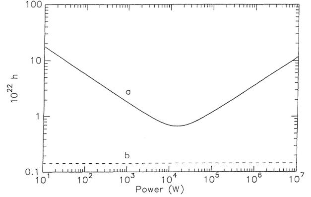
FIG. 3. (Curve *a*) The minimum possible gravitational wave amplitude  $h$  detectable as a function of power. (Curve *b*) The contribution of the mirror noise to  $h$ .
