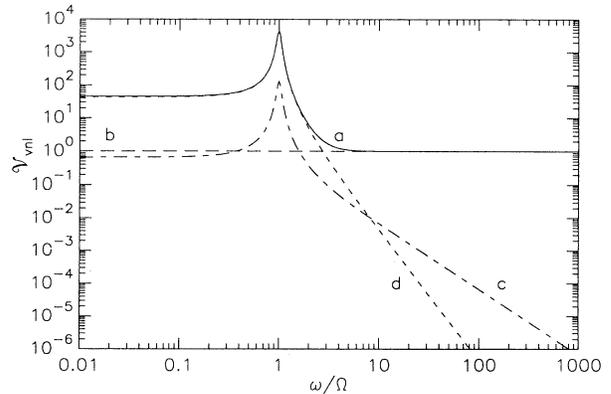
FIG. 2. (Curve *a*) The total noise,  $\mathcal{V}_{vnl}$  (solid line). Contributions to  $\mathcal{V}_{vnl}$ : (curve *b*) photon counting noise (dashed line); (curve *c*) mirror noise (dash-dotted line); (curve *d*) radiation pressure noise (dotted line).
