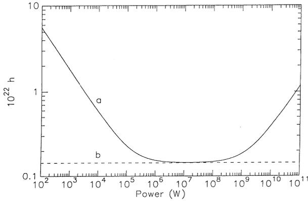
FIG. 8. (Curve *a*) The minimum possible gravitational wave amplitude  $h$  detectable as a function of power using a Kerr medium. (Curve *b*) The contribution of the mirror noise to  $h$ .
