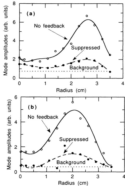
FIG. 4. Radial profiles of the mode amplitudes for the case of optimal suppression. (a)  $E \times B$  mode corresponding to the mode located at a frequency of 70 kHz. (b) ITG mode corresponding to the mode located at a frequency of 110 kHz.
