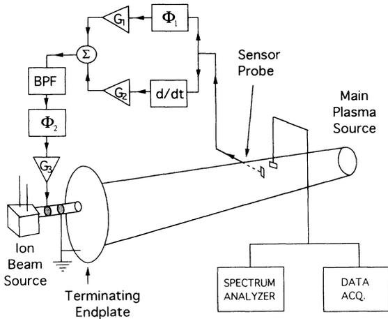
FIG. 2. Schematic of the feedback experimental setup for multimode control. A single feedback-modulated ion beam is the remote suppressor and a single Langmuir probe is the sensor. A second “scanner” Langmuir probe is used to monitor the fluctuations.
