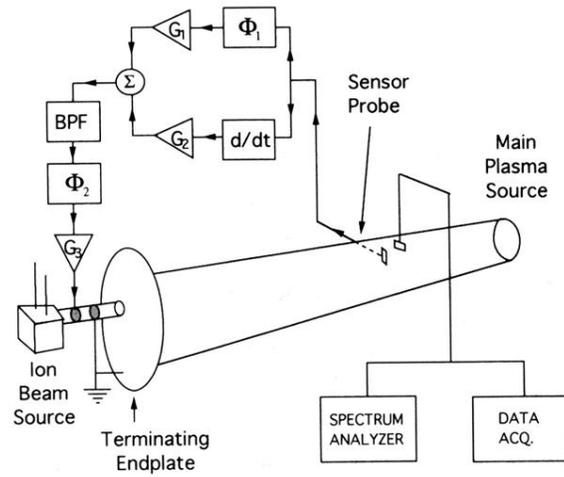
FIG. 2. Schematic of the feedback experimental setup for multimode control. A single feedback-modulated ion beam is the remote suppressor and a single Langmuir probe is the sensor. A second "scanner" Langmuir probe is used to monitor the fluctuations.
