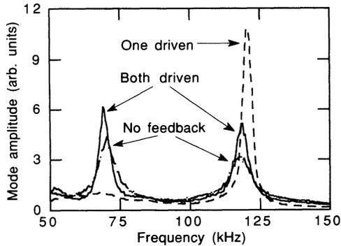
FIG. 5. Spectra for different combinations of feedback parameters: no feedback; both modes driven with  $G_R \sim 3.6$ ,  $\phi_{1R} \sim 90^\circ$ , and  $\phi_{2R} \sim 190^\circ$ ; and  $\eta_i$  mode driven while  $\mathbf{E} \times \mathbf{B}$  is suppressed.
