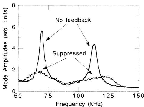
FIG. 3. Spectra of the mode amplitudes for the case of optimal suppression. The mode spectrum without feedback is also indicated.
