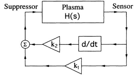
FIG. 1. Model of multimode feedback stabilization with a single sensor-suppressor pair. Another independent signal, representing another "state" of the plasma, is generated by differentiating the original signal.
