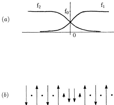
FIG. 7. The odd and even components for the soliton solutions (35) (a) and the diagrammatic representation of the whole localized structure in a monoatomic chain (b).
