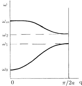
FIG. 1. Dispersion curves of a linear diatomic chain. “Acoustic” (the lower curve) and “optical” (the upper curve) branches are separated by the gap  $\Delta\omega = \omega_2 - \omega_1$ ,  $\omega_{1,2}$  being defined in Eq.(6).
