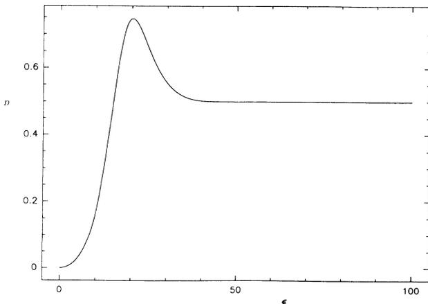
FIG. 1. Diffusion coefficient  $D$  vs perturbation parameter  $\epsilon$  for the case of  $V(\theta) = \sqrt{2} \cos(\theta)$ . The quasilinear estimate is  $\frac{1}{2}$ . Gaussian case with mean  $a = 0.09$  and standard deviation  $\sigma = 0.08$ .
