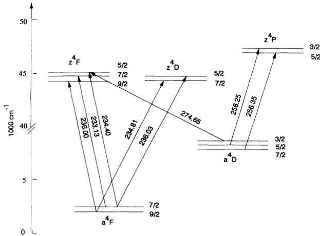
FIG. 1. Energy diagram showing the wavelengths (in nm) used to excite the quartet levels of Fe II studied here.
