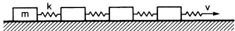
FIG. 1. Mechanical model consisting of a chain of blocks on a frictional surface. The blocks are connected by coil springs and the chain is pulled at one end with a small constant velocity.
