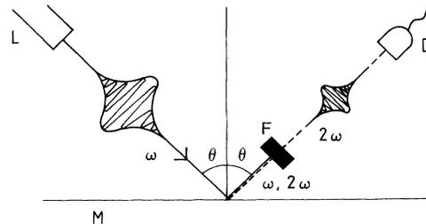
FIG. 1. A schematic diagram for second-harmonic generation.  $L$ , laser;  $M$ , nonlinear medium;  $F$ , filter to block the fundamental frequency; and  $D$ , detector.
