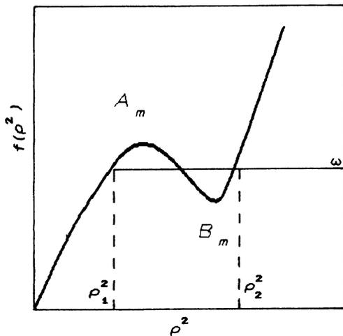
FIG. 1. The model  $f(I)=I-bI^3+cI^5$ .  $A_m$  and  $B_m$  are extrema of  $f(I)$ . Values  $\rho_1^2$  and  $\rho_2^2$ , which are the crossing points of the graph with the level  $\omega$ , are evidence of the two appropriate backgrounds.
