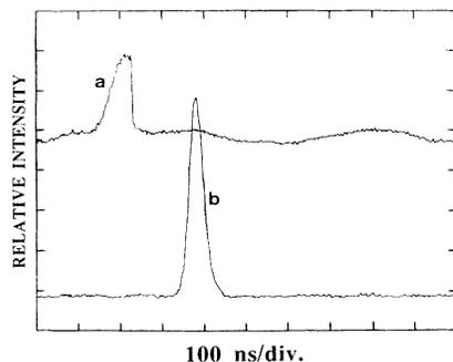
FIG. 3. The shape of the driving pulse (a) and that of the superfluorescence pulse (b) at a pressure of 0.1 Torr for the molecular vapor in the cell.
