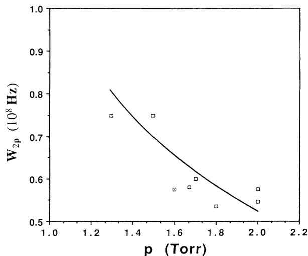
FIG. 5. The frequency of the fluctuation in dependence on the pressure of the vapor in the cell. The solid curve is the result of the calculation according to Eq. (2). The squares are the results of the measurement.
