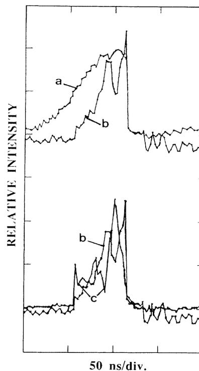
FIG. 4. The pulse shape of the driving beam before entering the cell (a); the pulse shape of the driving beam after propagation through the cell (b); and the pulse shape of the far-infrared superradiance pulse (c) if simultaneous interaction of the induced far-infrared radiation and the driving beam takes place with a  $\Lambda$ -like three-level system. The  $\text{NH}_3$  pressure in the cell is 1.7 Torr.
