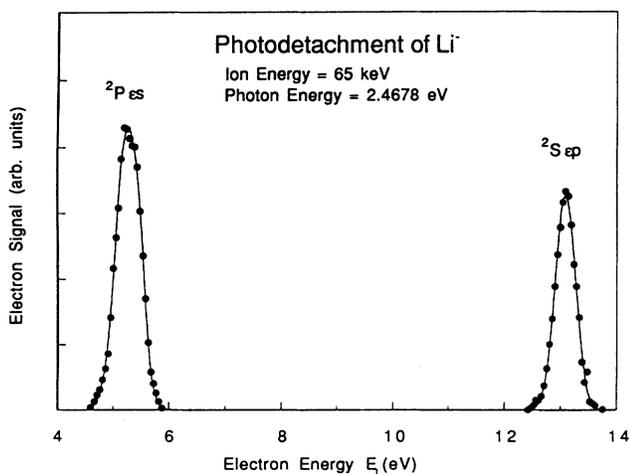
FIG. 1. Spectrum of photoelectrons detached from a fast beam of  $\text{Li}^-$  ions by visible radiation from a pulsed laser. The lower-energy and higher-energy peaks are associated with photodetachment via the  ${}^2P\epsilon s$  and  ${}^2S\epsilon p$  channels, respectively. In the ion frame the  ${}^2P\epsilon s$  channel threshold electrons have an energy of 2 meV. This is kinematically "amplified" to about 5 eV in the laboratory frame.
