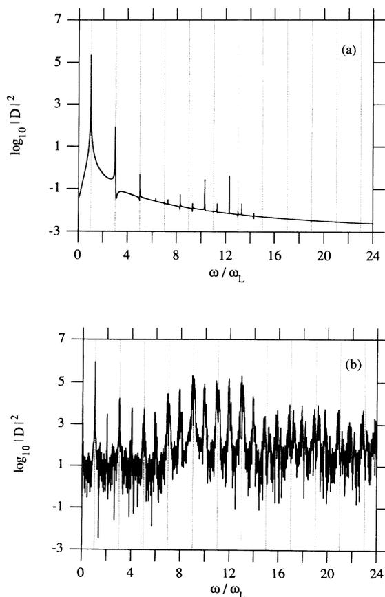
FIG. 5. Power spectra  $D(\omega)$  of the dipole  $\mu_z$  for two particular trajectories with  $\omega_L = 0.086$  a.u. and  $F_0 = 0.11$  a.u. For (a) the plane of the initially circular trajectory is perpendicular to the laser polarization, while for (b) it is parallel to the laser polarization.
