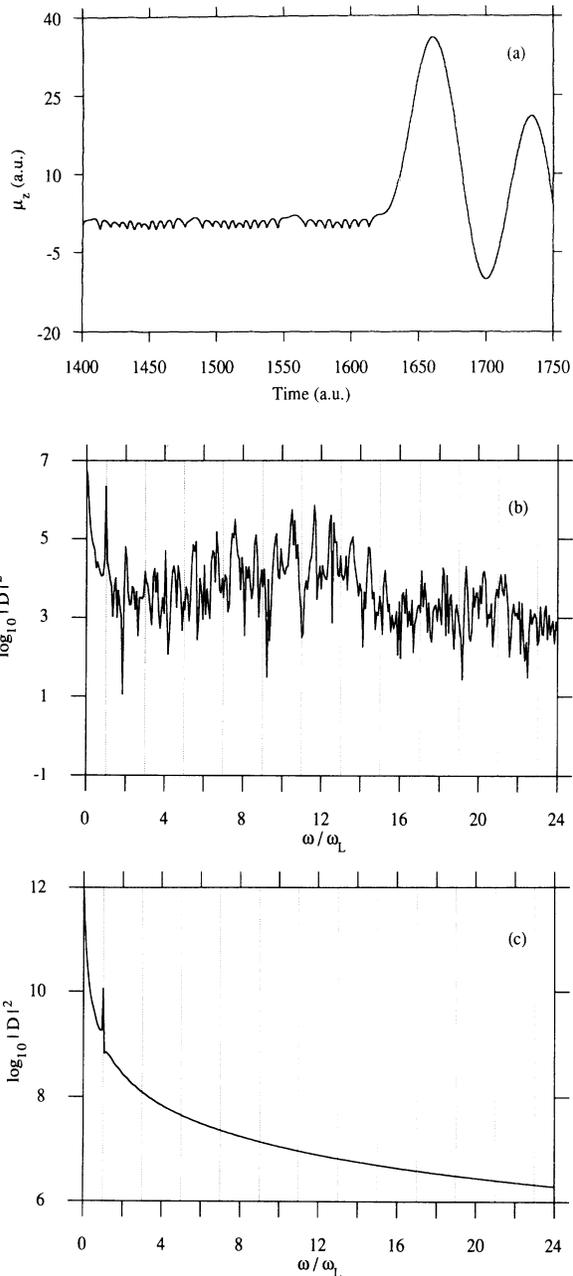
FIG. 6. (a) Temporal variations of the atomic dipole moment  $\mu_z$  of an ionizing trajectory, with  $\omega_L = 0.086$  a.u.,  $F_0 = 0.15$  a.u. Ionization takes place at approximately  $t \approx 1600$  a.u. (b) shows the power spectrum  $D(\omega)$  of  $\mu_z$  corresponding to the bound motion of the trajectory, i.e.,  $t < 1600$  a.u., while (c) shows the power spectrum corresponding to the unbound motion, i.e.,  $t > 1650$  a.u.
