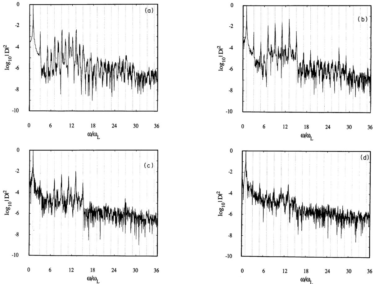
FIG. 8. Harmonic spectrum of a ground-state hydrogen atom in a laser field:  $\omega_L=0.086$  a.u., 2400 Monte Carlo trajectories were used. (a)  $F_0=0.11$  a.u. (b)  $F_0=0.12$  a.u. (c)  $F_0=0.13$  a.u. (d)  $F_0=0.14$  a.u.
