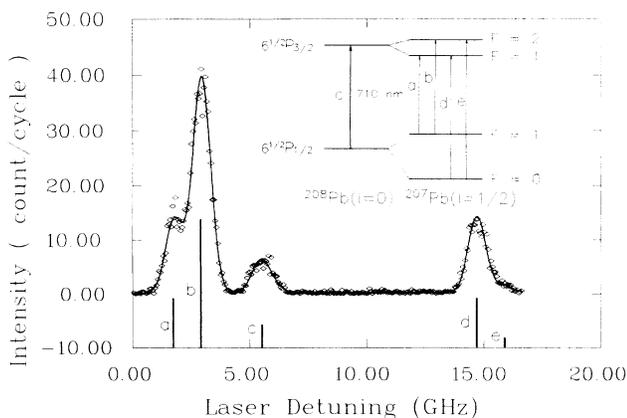
FIG. 2. Laser scan of the  $6P_{3/2}-6P_{1/2}$  fine-structure transition in  $\text{Pb}^+$  at 710 nm. The resonances *a*, *b*, and *d* are hyperfine components from  $^{207}\text{Pb}^+$  and *c* is from a contamination of  $^{208}\text{Pb}^+$ . The data are the average of ten consecutive scans. The Doppler limited linewidth corresponds to an ion temperature of 1600 K. The solid line consists of Gaussian functions fitted to the experimental points by a least-squares method.
