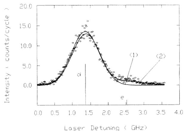
FIG. 4. Laser scan of the  $F=0-F'=1$  hfs component in the  $6P_{1/2}-6P_{3/2}$  fine-structure transition in  $^{207}\text{Pb}^+$ . From the comparison of one (1) and two (2) Gaussian functions fitted to the experimental points an additional component (*e*) is obvious, which we attribute to a weak admixture of an electric quadrupole allowed  $F=0-F'=2$  radiation.
