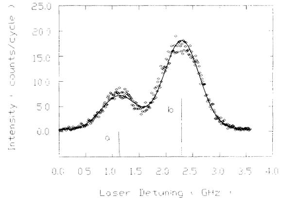
FIG. 3. Laser scan of the  $F=1-F'=1$  (*a*) and  $F=1-F'=2$  (*b*) hfs components in the  $6P_{1/2}-6P_{3/2}$  fine-structure transition in  $^{207}\text{Pb}^+$  at reduced potential depth. The linewidth corresponds to an ion temperature of 1027 K. Two Gaussian functions are fitted to the experimental points.
