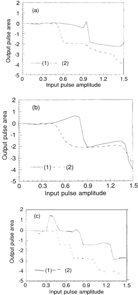
FIG. 8. Pulse area transmission as a function of the input amplitude  $A$  for the resonant case where dampings terms are included: (a)  $\gamma'\tau'=0.1$ , (b)  $\gamma'\tau'=0.05$ , and (c)  $\gamma'\tau'=0.01$ . The vertical axis is scaled in multiples of  $\pi$ .
