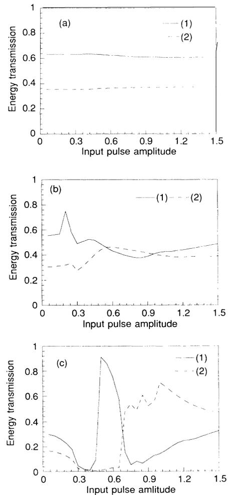
FIG. 6. Energy transmission normalized to the input energy as a function of the input amplitude  $A$  for the off-resonant case. Three different detunings are considered: (a)  $\Delta = 1$ , (b)  $\Delta = 0.5$ , and (c)  $\Delta = 0.1$ ; for small detunings only the system acts as a SIT soliton switch, while for large detunings the device behaves linearly. The input pulse duration was  $\tau' = 2$  and the coupler parameters are the same as those of Fig. 1.
