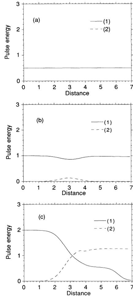
FIG. 1. Energy evolution vs distance  $\zeta$  of three different  $2\pi$  solitons: (a)  $A = 0.25$ ,  $\tau' = 4$ ; (b)  $A = 0.5$ ,  $\tau' = 2$ ; and (c)  $A = 1$ ,  $\tau' = 1$ , through the dual-channel directional coupler whose parameters are  $K = 2$ ,  $d = 1$ ,  $\zeta_m = 3$ ,  $\zeta_{\text{out}} = 7$ . The solid and dashed curves correspond respectively to the bar (1) and cross (2) channels of the NLDC. The curve relative to the cross channel in (a) coincides with the abscissa.
