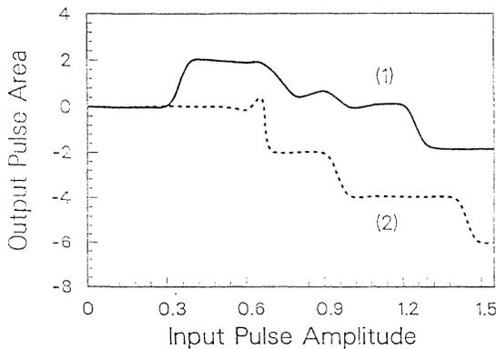
FIG. 5. Output pulse area vs input pulse amplitude for excitation of the NLDC on channel (1). The pulse was launched in channel (1) and the duration was  $\tau' = 2$ . The vertical axis is scaled in multiples of  $\pi$ . The area transmission exhibits a digital behavior. The coupler parameters are the same as those reported in Fig. 1.
