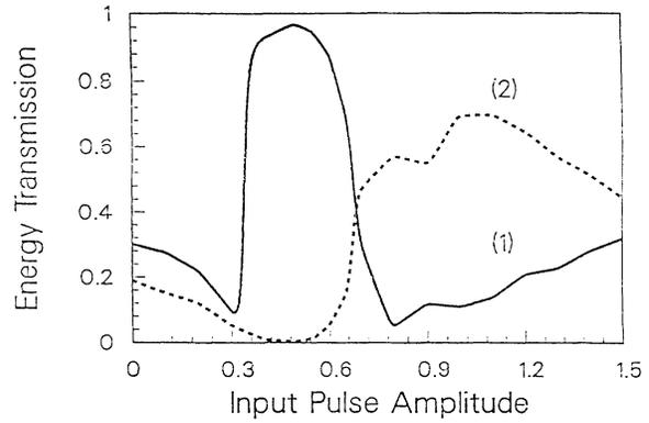
FIG. 3. Energy transmission normalized to the input energy for channels (1) and (2) as function of the amplitude  $A$ . The pulse was launched in channel (1) and the duration was  $\tau'=2$ . The parameters of the directional coupler are the same as those reported in Fig. 1.
