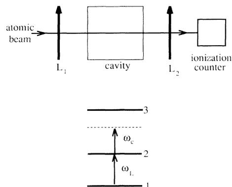
FIG. 1. Schematic representation of the QND scheme to measure the photon number in the cavity.  $L_1$  is a field used to prepare the state of the atoms so that they have a nonzero dipole on entering the cavity, while  $L_2$  ensures that the final ionization count will give information on the photon number in the cavity.
