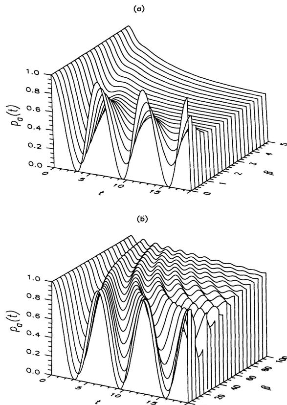
FIG. 5. A plot of the survival probability vs time for the case of Poisson injected probe atoms, with different injection rates. (a)  $\theta = \pi/2$ , (b)  $\theta = 0.01$ .
