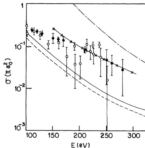
FIG. 4. Total capture cross sections ( $\pi a_0^2$ ) in  $e^+$ -He scattering: —, present; ---, FBA; - · - · -, second-order Faddeev-Watson (Ref. [9]); ×× Ref. [7]; †, Ref. [3]; ‡, Ref. [2].
