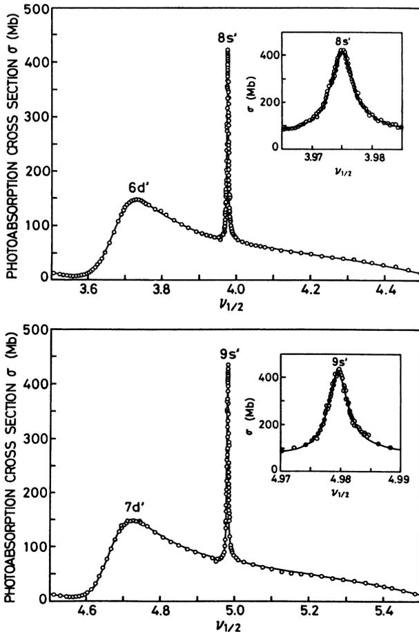
FIG. 1. Photoabsorption cross sections  $\sigma$  are plotted as a function of  $\nu_{1/2}$ .  $\circ$ , the present measurement; solid lines, the results of the curve fit with Eqs. (1) and (2).
