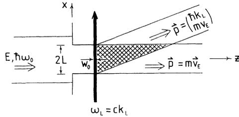
FIG. 2. Scattering of a two-level atom from a traveling-wave laser field. (Note the width of the laser is not drawn to scale; actually  $W_0 \gg 2L$ .) The shaded area represents the overlap region.
