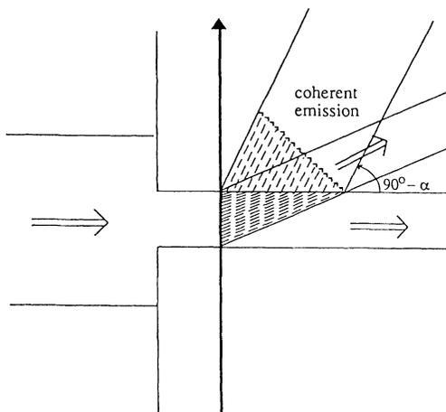
FIG. 5. The coherent radiation emitted from the two-level atom is depicted. The lengths of the arrows represent the amplitude of the radiation.
