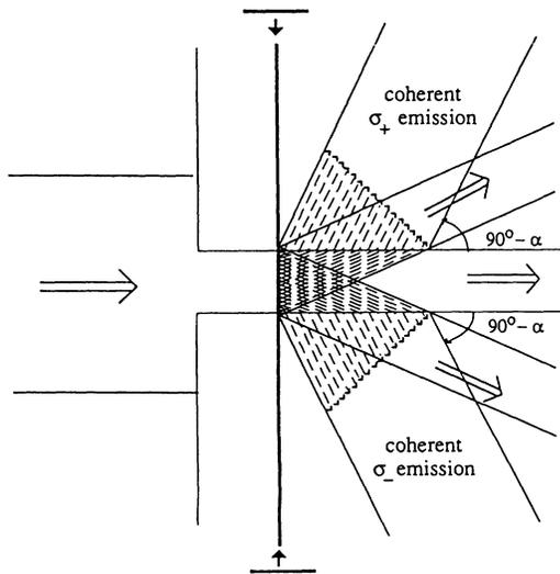
FIG. 6. The coherent radiation from the three-level atom is depicted. The lengths of the arrows represent the amplitude of the radiation of the two components corresponding to  $\sigma_+$  and  $\sigma_-$  polarizations.
