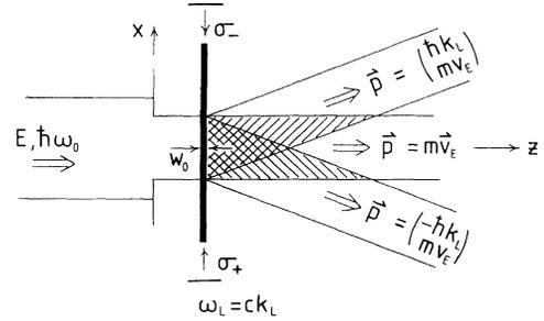
FIG. 3. Scattering of a three-level atom from a standing-wave laser field with  $\sigma_+ - \sigma_-$  counterpropagating (again the width of the laser is not drawn to scale; actually  $W_0 \gg 2L$ ). The shaded area represents the overlap region.
