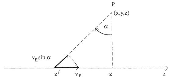
FIG. 4.  $V_E$  is the velocity of the atom in the  $z$  direction. The component of the velocity in the direction of the coherent radiation is  $V_E \sin\alpha$ .  $P$  is the position of the detector. The frequency of the light emitted by the atom in its rest frame is  $\omega_0$ . However, due to the Doppler shift, the frequency seen by the vector is the laser frequency  $\omega_L$ .
