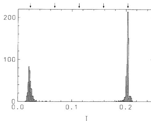
FIG. 4. Histogram of the final action values of the trajectories after the pulse [see Fig. 3(g)]. The arrows indicate the actions which semiclassically yield the bound states of a quantum-mechanical Morse oscillator modeling an O—H bond.
