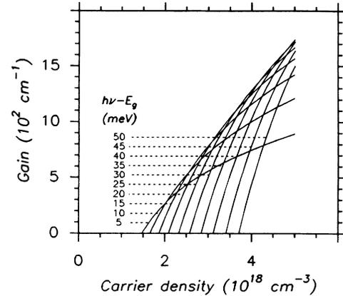
FIG. 1. Calculated gain coefficient  $g$  of  $\text{Al}_x\text{Ga}_{1-x}\text{As}$  as a function of carrier density for different photon energies  $h\nu$  relative to the  $\text{Al}_x\text{Ga}_{1-x}\text{As}$  band gap  $E_g$ . The laser parameters used for the calculation of all figures are given in Table I.
