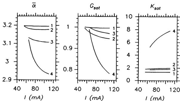
FIG. 6. Calculated values of  $\bar{\alpha}$ ,  $G_{sat}$ , and  $K_{sat}$  as a function of injection current for four lasers with different facet reflectivities (in percent): 1: 30-30; 2: 10-90; 3: 10-10; and 4: 1-100. The threshold currents lie at the starting point of each curve. Except for the 1-100 laser the averaged quantities depend only slightly on injection current.
