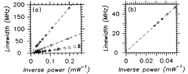
FIG. 7. (a) The circles show the calculated linewidth vs inverse output power for the same lasers as in Fig. 6. The dashed curves represent a linear fit. For all four lasers, the slope of these curves equals the slope predicted by the theory without saturation within 0.2%. (b) Enlarged section in the region of high output power for the 1-100 laser. The intercept shows a power-independent contribution of  $1.1 \pm 0.3$  MHz, apparently due to the effect of saturation.
