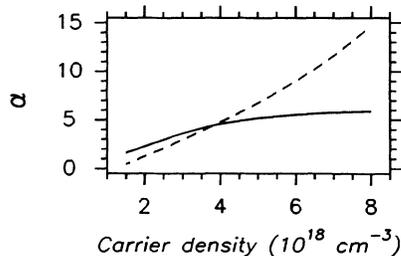
FIG. 3. The solid curve shows the calculated value of  $\alpha$  as a function of carrier density at fixed photon energy  $E=E_g+30$  meV. The dashed curve shows the (approximate) analytical expressions of Westbrook and Adams.
