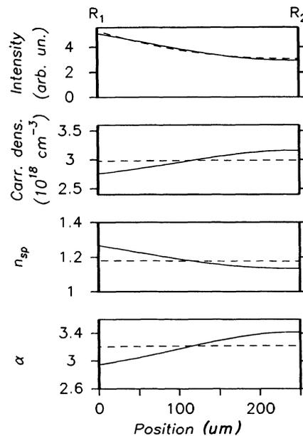
FIG. 5. Calculated intensity, carrier density, spontaneous-emission factor  $n_{sp}$ , and linewidth-enhancement factor  $\alpha$  as a function of the axial coordinate inside the laser.  $R_1=10\%$ ,  $R_2=90\%$ . The dashed curve corresponds to  $I=I_{th}$  (no saturation) and the solid curve to  $I=1.5I_{th}$ .
