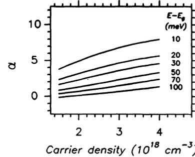
FIG. 4. Calculated value of  $\alpha$  as a function of carrier density  $N$  for different photon energies  $E$  relative to the band gap  $E_g$ .
