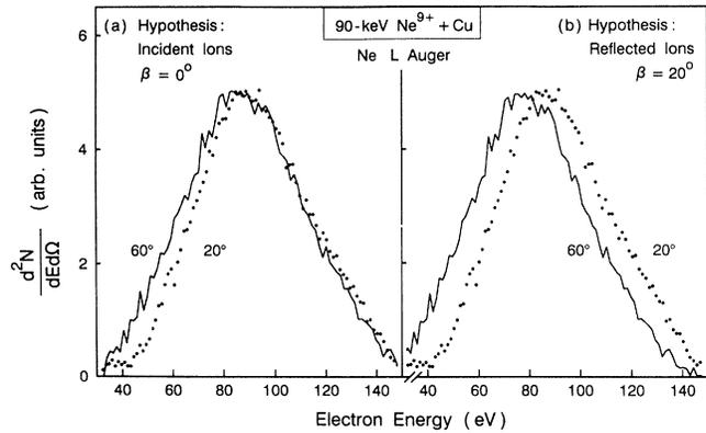
FIG. 3. Neon  $L$  Auger spectra produced by 90-keV  $\text{Ne}^{9+}$  incident under  $10^\circ$  on a Cu surface. Observation angles are  $\theta = 20^\circ$  and  $60^\circ$  as indicated. The continuous background is subtracted. The spectra are transformed to the projectile rest frame under the hypothesis that electrons are ejected (a) from incident ions and (b) from ions deflected by the surface under  $\beta = 20^\circ$  corresponding to specular reflection.
