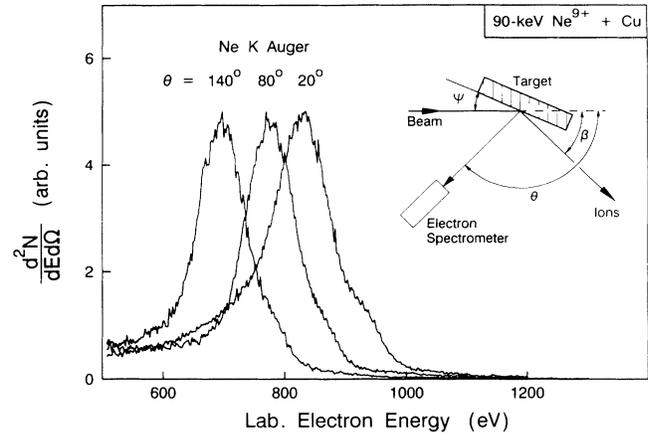
FIG. 1. Neon *K* Auger spectra for three different observation angles  $\theta$  with respect to the incident beam direction. The spectra are normalized to the same height. The angle of incidence is  $\psi=10^\circ$ . The scattering angle is labeled  $\beta$ .
