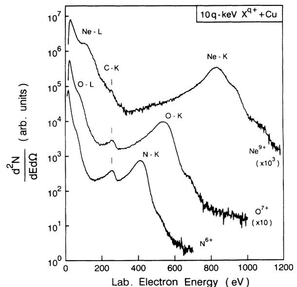
FIG. 2. Electron spectra produced in collisions of 60-keV  $\text{N}^{6+}$ , 70-keV  $\text{O}^{7+}$ , and 90-keV  $\text{Ne}^{9+}$  on a Cu surface under the incidence angle of  $\psi=10^\circ$ . The electron-energy scale refers to the laboratory rest frame. Electron observation angle is  $\theta=20^\circ$  with respect to the incident-beam direction.
