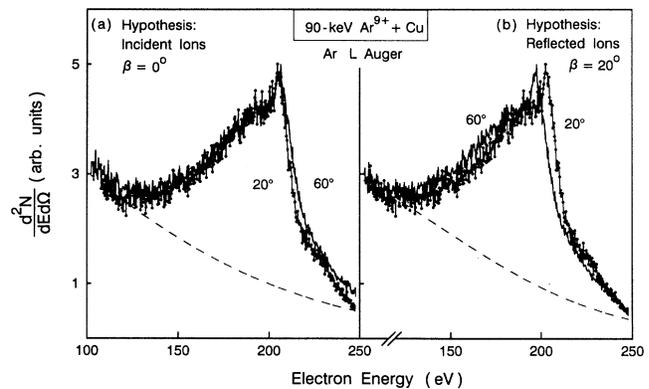
FIG. 4. Argon  $L$  Auger spectra produced by 90-keV  $\text{Ar}^{9+}$  incident under  $\psi = 10^\circ$  on a Cu surface. Observation angles are  $\theta = 20^\circ$  and  $60^\circ$ . The spectra are transformed to the projectile rest frame under the hypothesis that electrons are ejected (a) from incident ions and (b) from ions deflected by the surface under  $\beta = 20^\circ$ . Energy resolution is 0.5%.
