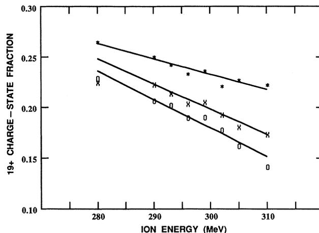
FIG. 3. The  $\text{Ti}^{19+}$  charge-state fraction for all (\*), better (X), and best (O) channeled ions (see text) vs ion energy. The straight lines through the points are the results of linear least-square fits to the data points. The vertical extent of the symbols in this figure and Figs. 4 and 5 represents the statistical error bars of the data.
