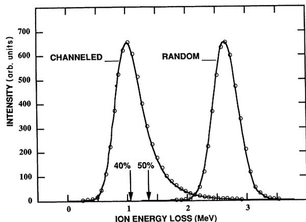
FIG. 2. Energy-loss spectrum of channeled ions (peak at 1.09 MeV) and ions traversing the Au crystal in a random direction (peak at 2.67 MeV). The location of the energy cuts made at  $0.4E_f$  and  $0.5E_f$  are shown as arrows on the abscissa.
