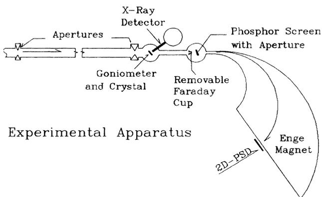
FIG. 1. Sketch of the apparatus. The Ti ions enter the apparatus from the left and terminate their flight at the focal plane of the Enge magnet (2D-PSD means a two-dimensional position-sensitive channel-plate detector).
