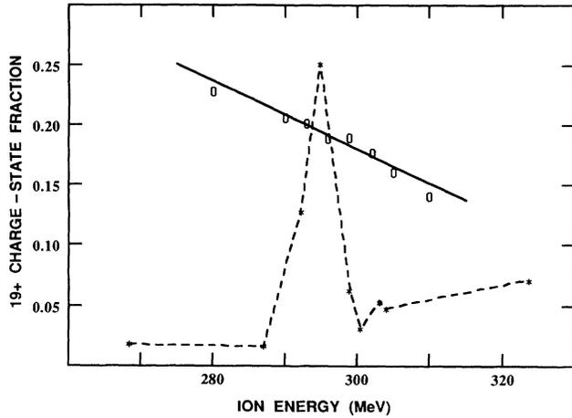
FIG. 4. The 19+ charge-state fractions of the best channeled ions of Ref. [13] (\*) and this work (O) vs ion energy. The data of Ref. [13] are connected by a dashed line. The line through the data of this work is the same as in Fig. 3.
