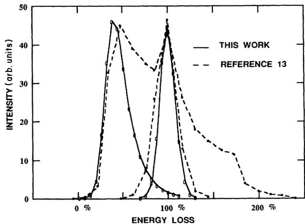
FIG. 6. Channeled and random energy-loss spectrum of ions with exit charge state 19+ plotted as a percentage of the mean energy loss of ions traversing the Au crystal in a random direction. Data of this work (O) scaled to  $E_r$  with a solid line connecting the points. Data (\*) from Fig. 1(d) of Ref. [13] scaled to the appropriate  $E_r$  with a dashed line connecting the points. Both sets of data were taken with a 293-MeV  $\text{Ti}^{20+}$  ion beam entering the crystal.
