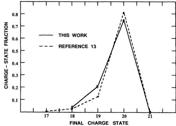
FIG. 5. Exit charge-state fractions for 293-MeV  $\text{Ti}^{20+}$  channeled along the  $\langle 100 \rangle$  axis of a 1520-Å-thick Au crystal as measured in this work (O) and the data (\*) for well channeled ions from Fig. 2 of Ref. [13].
