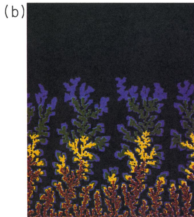
FIG. 1. Digitized images from (a) the separating plates experiment and (b) associated computer simulation. Plate dimensions in (a) are approximately 9\text{ cm} \times 9\text{ cm} , initial separation between the plates is 0.05\text{ mm} . The rate of separation at the lifted end is 0.025\text{ cm/min} .
