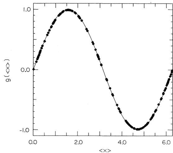
FIG. 2. Comparison between the function  $g(\langle x \rangle_m) = (\langle x \rangle_{m+1} - 2\langle x \rangle_m + \langle x \rangle_{m-1})/(2kT)$ , computed for the chaotic trajectory of Fig. 1 (dots), and the kick function  $g = \sin x$  (solid line).
