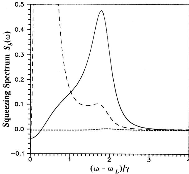
FIG. 7. Squeezing spectrum of the depleted pump,  $S_b(\omega)$ , for different widths of the external cavity. The solid curve corresponds to  $\Gamma_b=1$ , the long-dashed curve to  $\Gamma_b=0.1$ , and the short-dashed curve to  $\Gamma_b=10$ . Here  $G=0.5$  and the values of other parameters are the same as in Fig. 6. The frequency  $(\omega-\omega_L)$  is given in units of  $\gamma$ , i.e., one-half of the free-space atomic spontaneous emission width.
