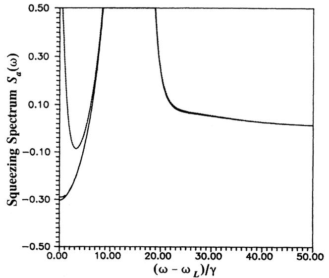
FIG. 5. Squeezing spectrum of the two-photon dressed-state laser,  $S_a(\omega)$ , corresponding to conditions of Fig. 4 and  $\Delta_2=8.5$ . Solid curve,  $G=0$ ; long-dashed curve,  $G=0.001$  (noticeable only around  $\omega-\omega_L=0$ ); short-dashed curve,  $G=0.01$ . The frequency  $(\omega-\omega_L)$  is given in units of  $\gamma$ , i.e., one-half of the free-space atomic spontaneous emission width.
