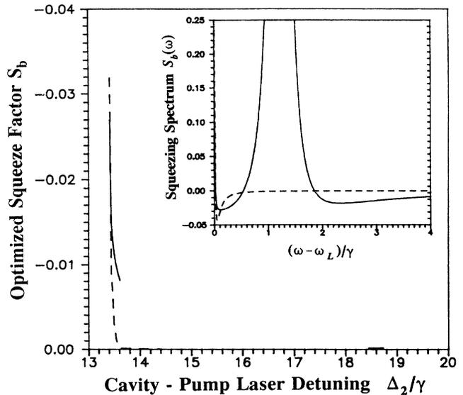
FIG. 2. Optimized squeeze factor  $S_b$  for the depleted pump vs  $\Delta_2$  and (inset) the pump squeezing spectra  $S_b(\omega)$  with  $\Delta_2$  fixed at 13.41. The solid and dashed curves are drawn for  $G=0.01$  and 0.001, respectively. Other parameters as in Fig. 1. The frequencies  $\Delta_2$  and  $(\omega-\omega_L)$  are given in units of  $\gamma$ , i.e., one-half of the free-space atomic spontaneous emission width.
