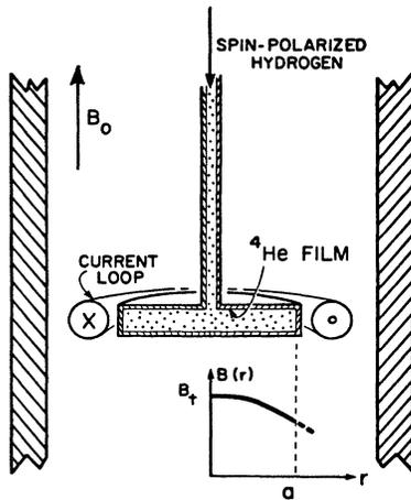
FIG. 2. Geometry for a two-dimensional trap for spin-polarized hydrogen. A gas of spin-polarized hydrogen is confined in a solenoid by the field  $B_0$ . Atoms in contact with the  $^4\text{He}$  surface produce a two-dimensional adsorbed gas that is trapped by the radial potential created by the field of the current loop  $B_t(r)$ .
