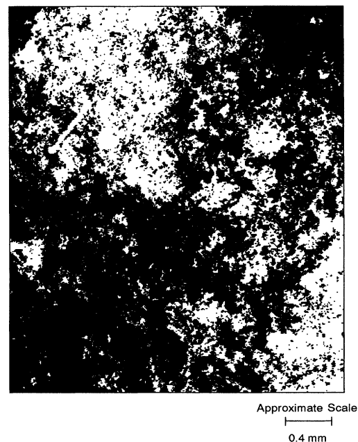
FIG. 3. Scanning electron micrograph of a metal cast of the flow paths in a fracture in granite rock. The pattern covers an area 4 \times 2 \text{ mm}^2 . The black regions are the metal. The pattern shows features at all length scales and has a fractal dimension D = 1.94 .
