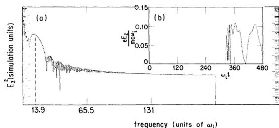
FIG. 1. Reflection from an overdense front. (a) The power spectrum of the reflected radiation. (b) The time history of the reflected radiation.
