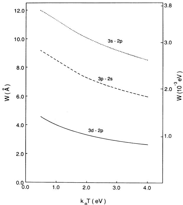
FIG. 3. Electron contribution to the linewidth for the components of  $H_\alpha$ . The electron density is  $10^{17} \text{ cm}^{-3}$ .
