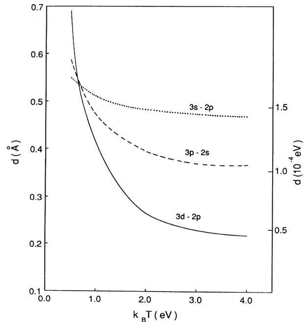
FIG. 2. Line shift  $d$  for the components of  $H_\alpha$ . The left scale gives the shift in  $\text{\AA}$ ; the right, in units of  $10^{-4} \text{ eV}$ . The electron density is  $10^{17} \text{ cm}^{-3}$ .
