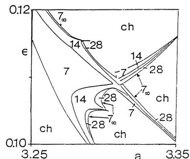
FIG. 5. Enlarged sector of Fig. 4. Details of the coalescence of two  $p=7$  windows in  $S$ . The boundaries  $7_\infty - ch$  mark transitions from period doubling to chaos. At the lines  $7 - ch$  intermittency appears.
