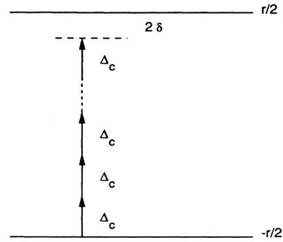
FIG. 2. Schematic diagram showing the system described by the effective Hamiltonian.
