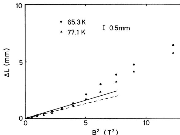
FIG. 3. Extension  $\Delta L$  of the gas-liquid interface as a function of a square of the applied magnetic field  $B^2$  at different temperatures, 65.3 and 77.1 K.
