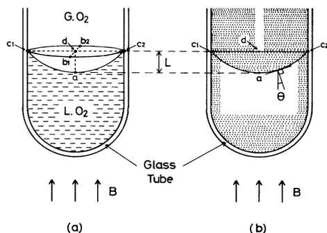
FIG. 2. An illustration of the gas-liquid interface in the applied magnetic field of 2 T, corresponding to the photo in Fig. 1(c).
