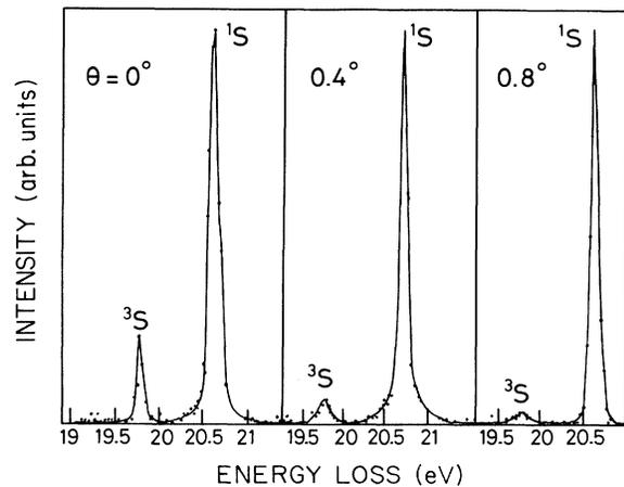
FIG. 4. Typical energy-loss spectra for the  $2^3S$  and the  $2^1S$  excitation in helium at scattering angles of  $0^\circ$ ,  $0.4^\circ$ , and  $0.8^\circ$  for 500-eV incident electrons. Intensity scale is normalized to the peak for the  $2^1S$  excitation.
