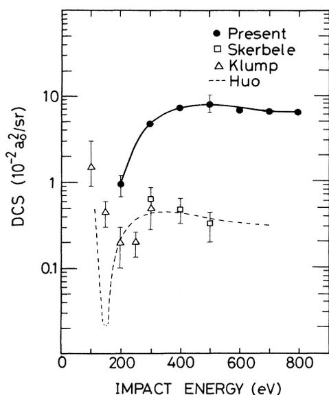
FIG. 6. Differential cross sections for the  $2^3S$  excitation in helium at  $\theta=0^\circ$  as a function of the incident electron energy. Corrections due to the limited angular resolution are not applied.
