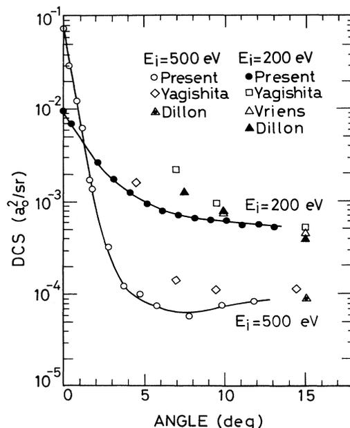
FIG. 5. Differential cross sections for the  $2^3S$  excitation in helium as a function of the scattering angle for the incident electron energies of 200 and 500 eV.
