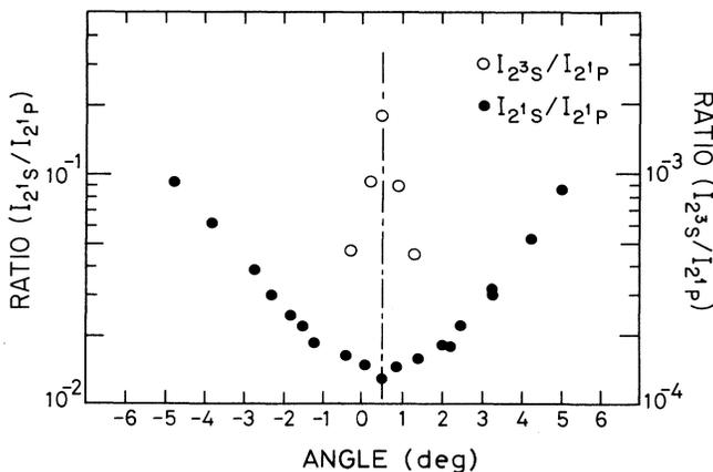
FIG. 3. Calibration of the zero angle position by means of the scattering symmetry of the DCS's for the  $2^1S$  and the  $2^3S$  excitation relative to the  $2^1P$  excitation. The incident electron energy is 500 eV.
