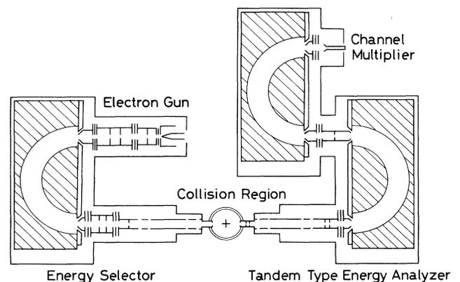
FIG. 1. Schematic diagram of the electron-energy-loss spectrometer with a tandem-simulated-hemispherical analyzer.
