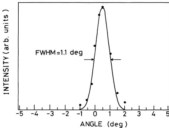
FIG. 2. Typical angular resolution of the apparatus.
